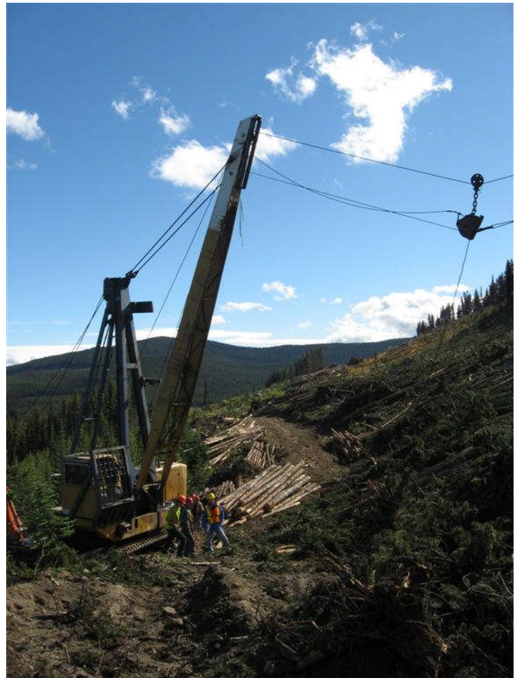
Specialized equipment, like this cable harvesting system, is used to protect more sensitive sites.
